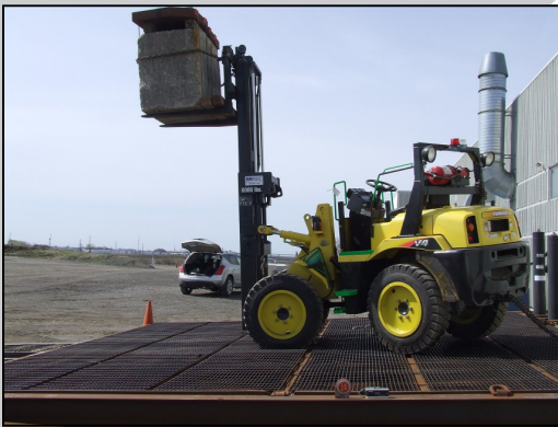
Our oscillating rear-axle contributes to best-in-class stability
