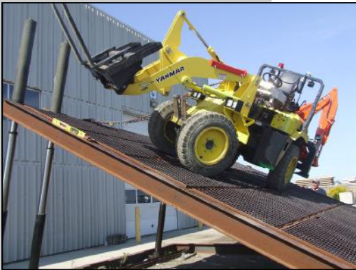
An oscillating rear axle ensures the unit stays stable, even in a tight turn.
